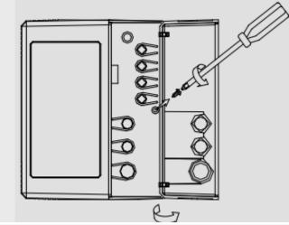
**3.** Grasp the case and wall plate separately by two hands and lift the thermostat up the wall plate from the right side (away from LCD)
