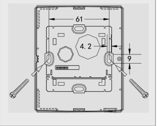
**7.** Mount the thermostat on the wall plate. Make sure all pins insert into the pinholes correctly.
